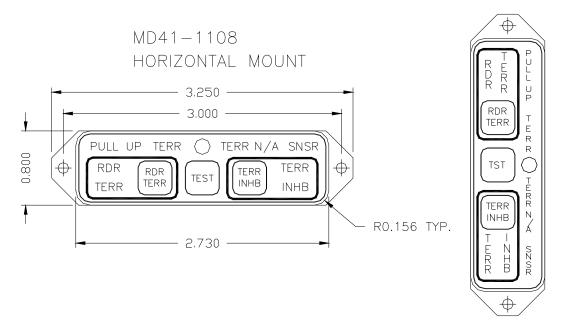
Note 1: Use two 4-40 X 3/8" Flat Head Phillips Screws for Mounting
